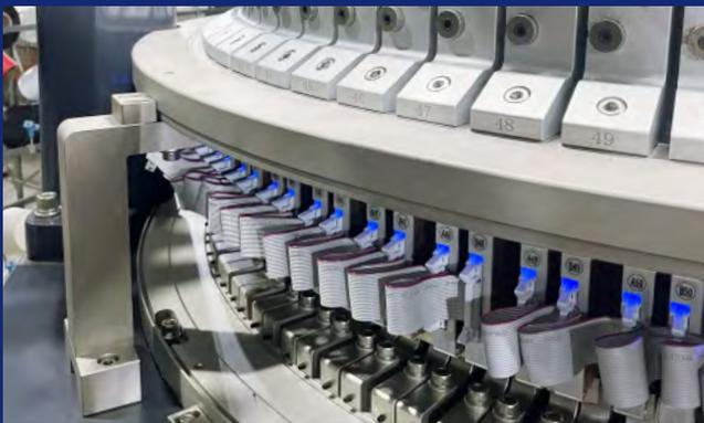
※ Cylinder Rib transfer jacquard machine knitted for garment & shoes fabrics both.
