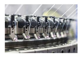
New developed type to meet varying changes in the market. This small-diameter knitting machine can produce seamless shirts, underwear, swimwear and so on. Gear and all important components are imported from Japan and German to ensure its stable performance. Groz-beckert needles are used to produce quality fabric and prolong the lifespan of machine.
