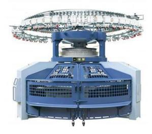
Following the gear design without unfolding the fabric, allows easy rolling up of cloth. Its safety shutdown device functions when the cloth is not cut completely.
