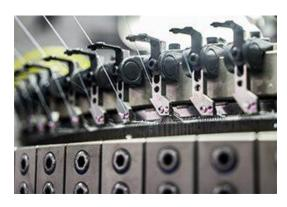
Widely used in high-volume production of soft and comfortable underwear fabric. Sintelli's main gear systems are all embedded in an oil bath to lubricate and prolong the lifespan of the gear system. All gears are fluted simultaneously to minimize backlash between dial and cylinder needles. Users can handle different fabric changes by choosing Sintelli's double series.
