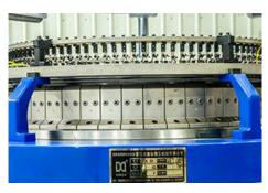
Can be configured into a machine for fleece yarn, tie-in yarn and back yarn for knitting fish scale, twill and French double fleece. The surface of the right-side of the cloth can be made into a velvet after fleece brushing. This 3-thread fleece machine offers high productivity because of the high number of feeders included, replacing older, obsolete models. The length of the wool yarn can
