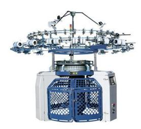
This 3-thread fleece machine offers high productivity because of the high number of feeders included, replacing older, obsolete models. The length of the wool yarn can be adjusted by changing the sinkers and cams.
