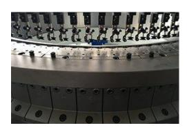
Reverse Plated Loop Single Circular Knitting Machine features different types of sinkers, which can knit towelling with differing heights of loops pile. This machine can feature reversed cams and normal cams respectively. With a cloth rolling system, it can evenly roll up fabrics without leaving folds.
