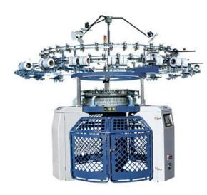
Reverse Plated Loop Single Circular Knitting Machine features different types of sinkers, which can knit to welling with differing heights of loops pile. This machine can feature reversed cams and normal cams respectively.
