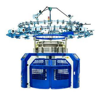
This machine manufactures loop pile or terry fabrics, which can be used for producing bath towels, to welling blankets, to welling pillows and other soft-cloth materials.
