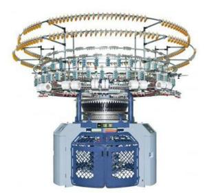
Based on the single knitting machine, the single striper knitting machine adds 4-color or 6-color striper knitting machine parts and a micro-computer control system.
