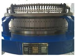
miss cams. High precision central raising and falling system can adjust the fabric weight conveniently and quickly. The special design of the feeding yarn carrier makes the option of Lycra more proficient. Featuring an ergonomic design, the additional middle feeding yarn transfer ring makes it easy for personnel to monitor and carry yarn, without the machine touching the operator's body; at the same time, the yarn carrying system is freer and steadier,
