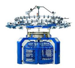
Designed with the central adjustment system to adjust fabrics in different levels of density easily and conveniently, normally equipped with different gauges of cylinders which is easy to alter and can meet the varying requirements in the knitting market.
